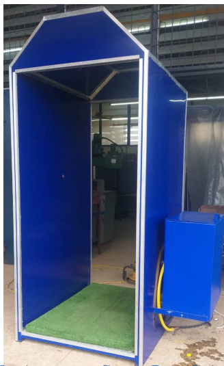
Figure 8: Automatic Spray Disinfectant Booth
